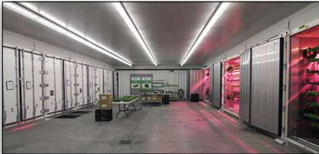
**The rotating shelving brings all plants to the front of the growing chamber regularly, eliminating the need for aisle access to reach the plants.** (IMAGES COURTESY CUBICFARMS)
